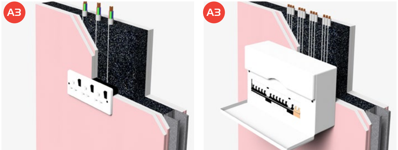
FZ100 Fire Safe Zone and gang socket box with twin and earth cables
